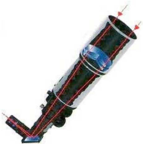
Schematic view of a Refracting Telescope
