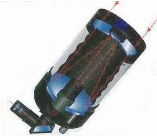
Schematic view of a Schmidt-Cassegrain
