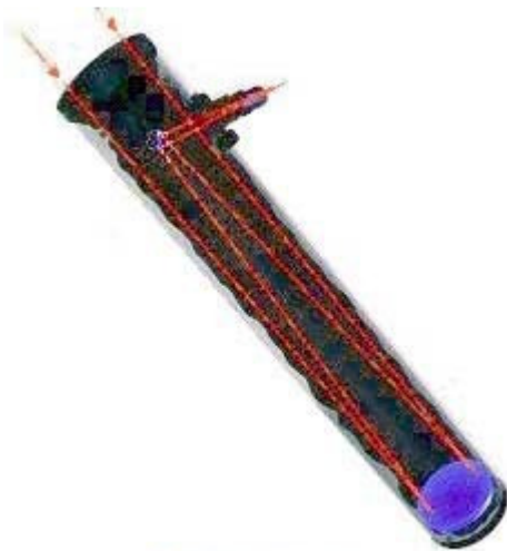
Schematic view of a Newtonian / Reflecting Telescope
