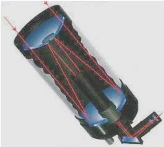
Schematic View of a Maksutov-Cassegrain
